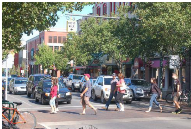
Figure 8: An elevated cross-walk supporting pedestrian oriented transportation
